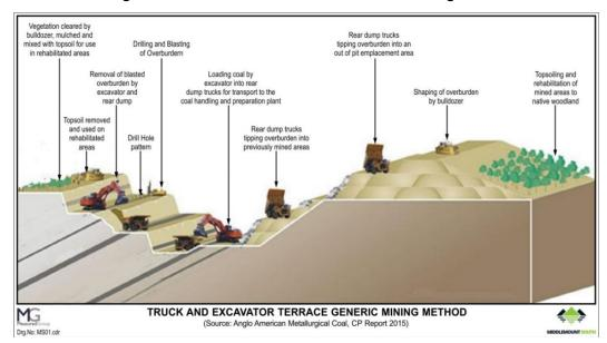
Figure 7: Truck and Excavator Terrace Generic Mining Method
